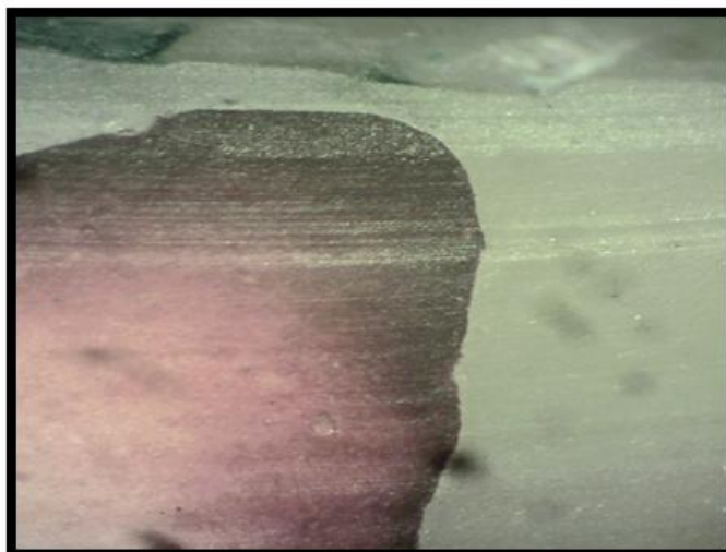
Fig. 8. Measuring marginal fit of VITA CAD temp (group A) PMMA provisional material under stereomicroscope.
