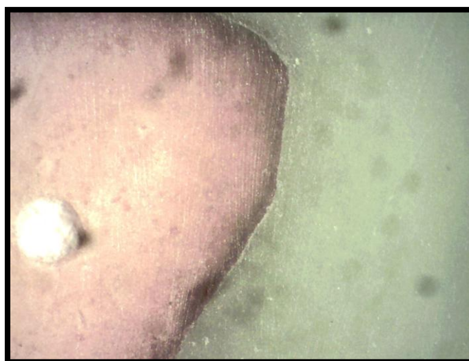
Fig. 9. Measuring marginal fit of TELIO CAD (group B) PMMA provisional material under stereomicroscope.
