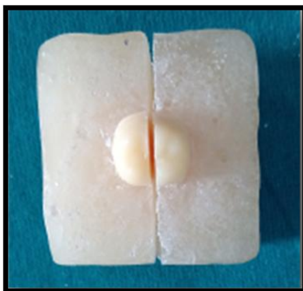
Fig. 7. Sectioning of samples embedded in acrylic resin
