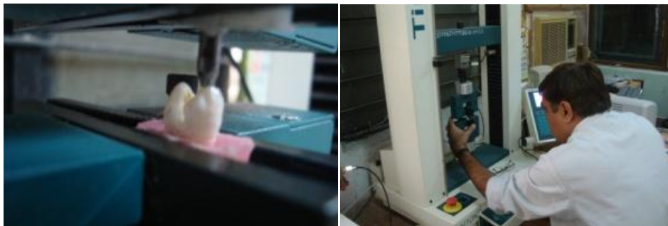
Figure 2: Mounted tooth in the acrylic cylinder under the LR5k testing machine.
