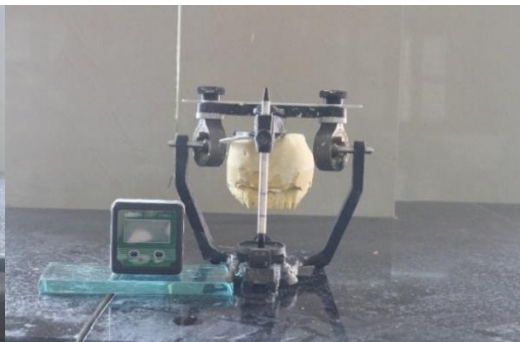
Fig 4. Mounted maxillary cast with digital protractor
