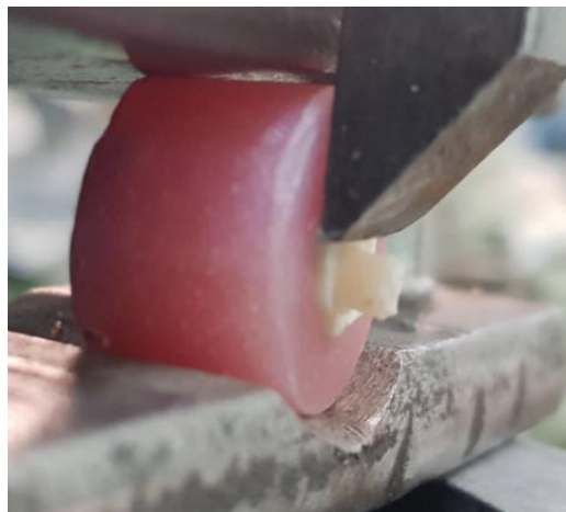
Fig. 8: Specimen subjected to load using chisel attachment
