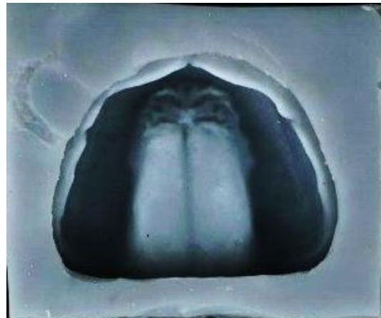
Figure 2, Mould used for epoxy resin cast fabrication.
