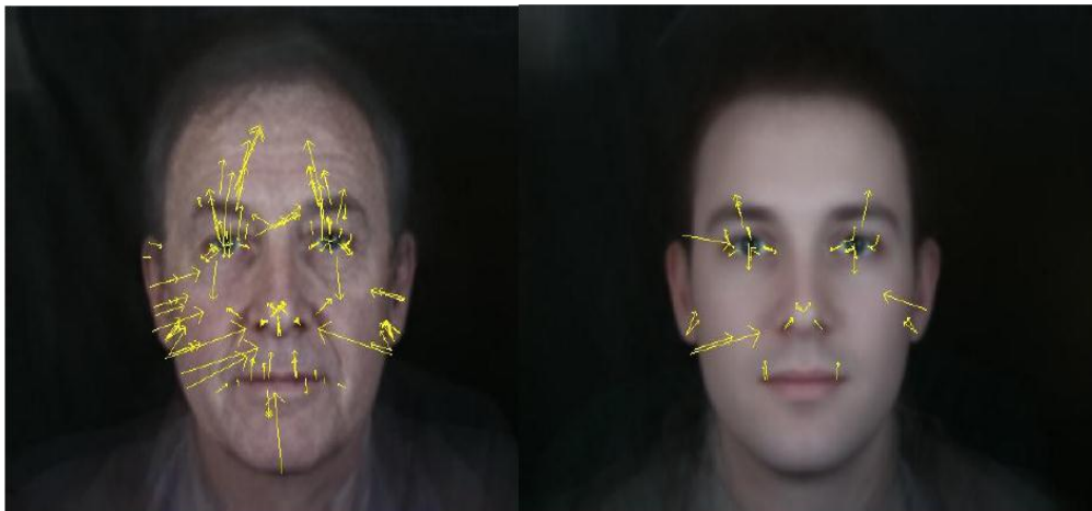
Fig 4: Keypoint vectors are drawn on the two men's face images. Most of the features appear on the eyes, nostrils, the top of nose, the corners of the mouth and the earlobes.
