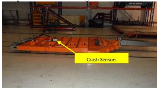
Figure 7. Sled test of vehicle frontal impact simulation.
