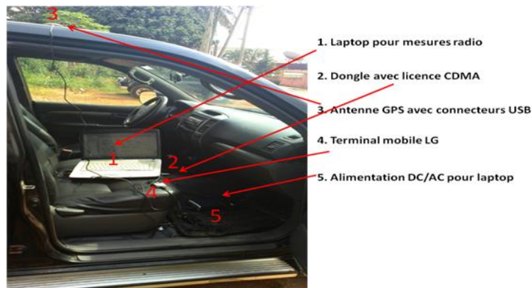
Figure 1: Drive test measurement kit installed on vehicle.
