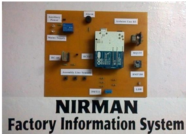
Fig. 14. Hardware Implementation of Data Acquisition System in NIRMAN FIS
