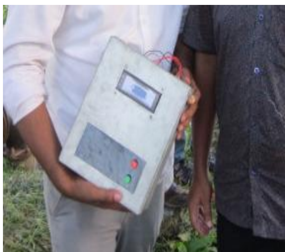
Fig. 7. Prototype 1 kV 100 A dc pre-paid smart energy meter.
