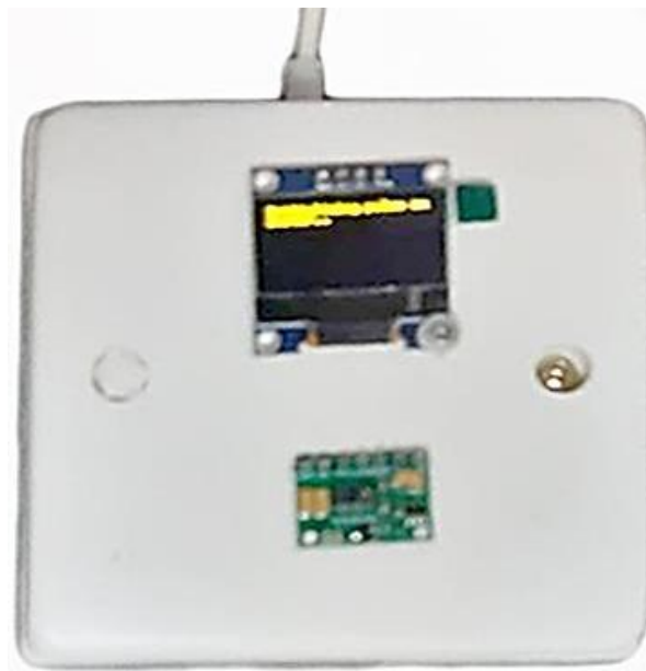
Figure 6: Real-time implemented pulse oxygen saturation level measuring device on a printed circuit board and enclosed in a casing
