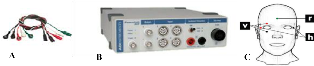
Fig (1) A: five electrodes, B: a powerlab (26T) device and C: the image demonstrates the placement of the EOG electrodes on the face
