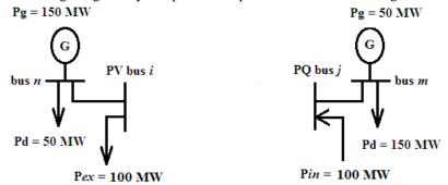
Fig. 4. Decoupled model of UPFC.
