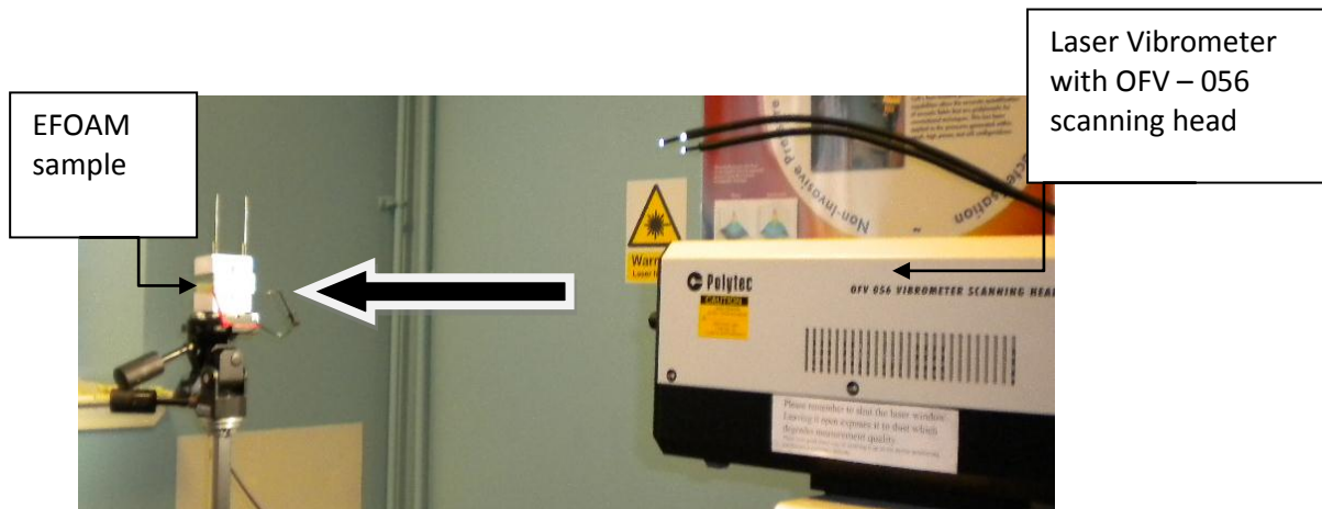
Fig.5. Measuring the inverse piezoelectric effect in the EFOAM sample
