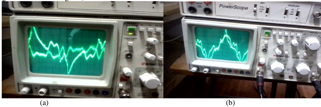
Fig.10 Waveform Observed (a) Without UPFC (b) With UPFC At Sending End For Injected Voltage And Current
