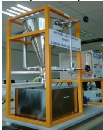
Fig.3. Conical Tank Level Process
