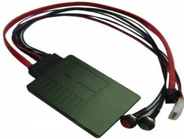
Fig 3.2 SSD with built-in data destruction
