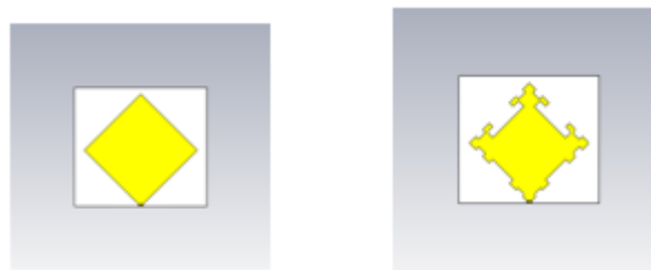
Figure 3(a) Square Patch Figure 3(b) 2 nd Iteration Fractal Figure 3 Corner feed to determine terminal impedance
