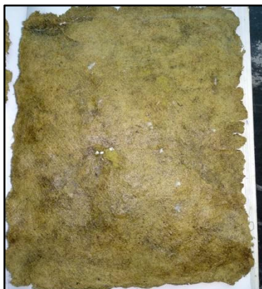
Figure 6: Banana leaf sheet after bioplastic coating
