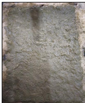
Figure 4: Processed Banana leaf pulp layered on mould and deckle
