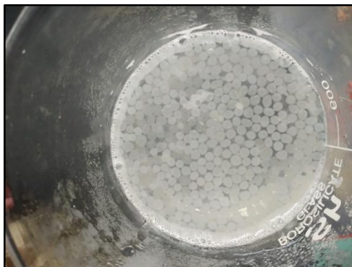
Figure 2: Xylanase enzyme immobilized in calcium alginate beads
