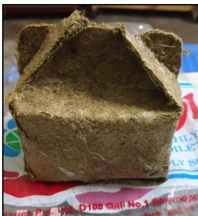
Figure 7: Banana leaf sheet made into packaging box
