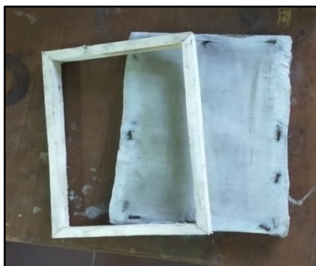
Figure 1: Mould and Deckle fabricated for this study
