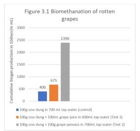
Figure 3.1 shows the bio methanation data of rotten grape juice and pomace compared to control (inoculum/Cow dung). 100 mL grape juice produced 675 mL biogas, while 100 mL grape pomace produced 2390 mL biogas in 10 days. The solid content of the pomace is responsible for high yield of gas this opens up new opportunity related to Bio processing use for production of biofuels like Biogas which can considerably reduce our present dependence on fossil fuels.
