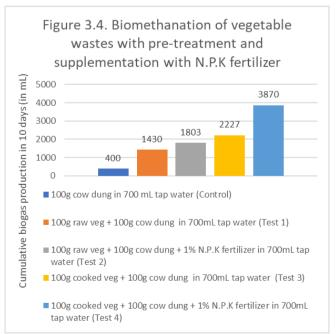
Figure 3.4 shows the Bio-methanation data of vegetables wastes. India is one of the leading producers of vegetables and fruits, where almost 30% of the produce goes wasted due to physical damages and lack of proper storage facilities. Fig 3.4 clearly shows biogas yield by 1430 mL without any addition, 1803 mL with supplementing N.P.K fertilizer, 2227 mL when it was pre-treated with steam and 3870 mL when it was pre-treated with steam along with N.P.K fertilizer supplementation.
