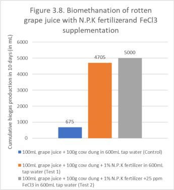
Figure 3.8 shows bio-methanation levels on supplementation with N.P.K fertilizer and FeCl<sub>3</sub> combination. With N.P.K fertilizer supplementation alone, 4705 mL gas was produced and additional supplementation of FeCl<sub>3</sub> could increase production to 5000 mL. This proves that supplementation of media with nitrogen potash and phosphorus, optimum concentration of substrates and FeCl<sub>3</sub> could improve biogas production from rotten grape juice.
