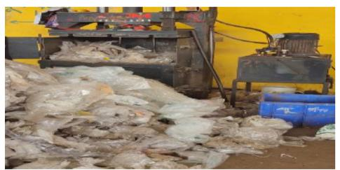
Fig. 4 - Plastic Compressing, bundling machine at MRF
