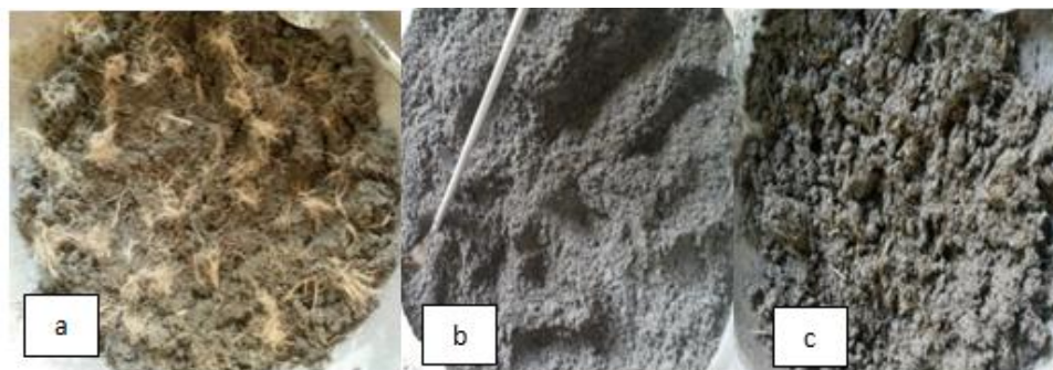
Fig.2.a. Cement, sands and filaments, b. Ash, c. Cement, sands, filament and ash was mixed,
