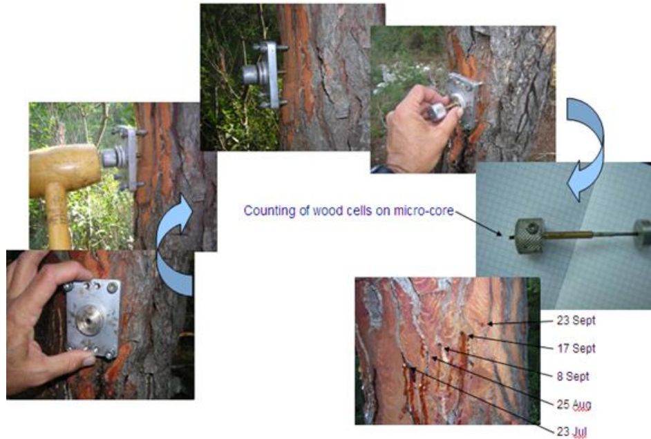
Figure 2. Determining the seasonal dynamic of cambial activity: periodic micro-samplings in the outer part of the trunk.
