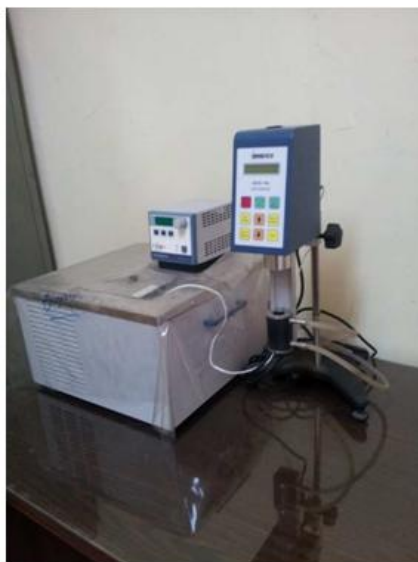
Figure-2: The Viscometer test device (Viscometer model DV-II (Spindle SC4-18/ Sample chamber SC4-13(p)) manufactured by a Brookfield company in the USA).
