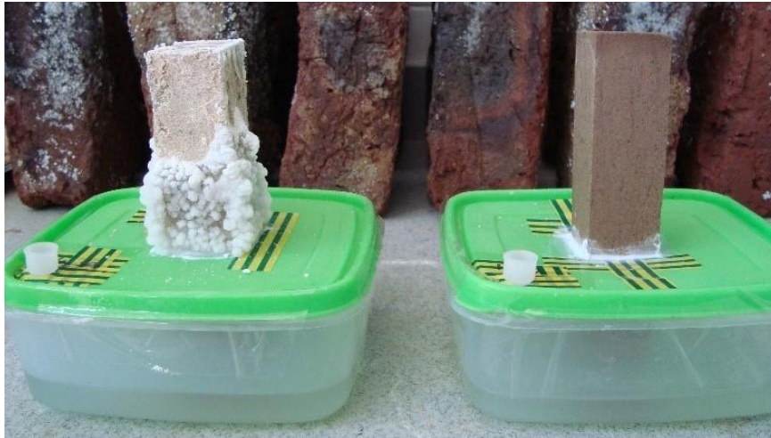
Fig. 1: Experiment on the effects of groundwater on sandstone sample showing surface salt crystallization (left) and potable water with little effect (right)
