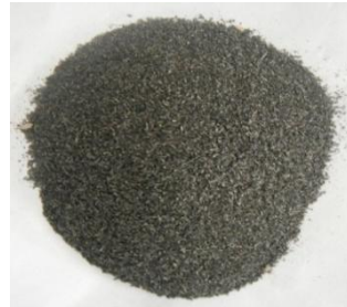
Plate 3: 600µm aggregate sizes of iron filings
