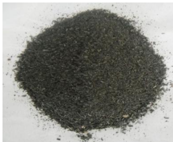
Plate 4: un-sieved aggregate of iron filings
