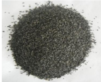
Plate 2: 1.18mm aggregate sizes of iron filings
