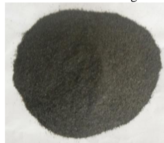
Plate 5: 300µm aggregate sizes of iron filings
