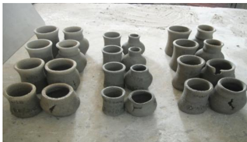
Plate 9: Outcomes of throwing of clay and iron filings at green ware stage
