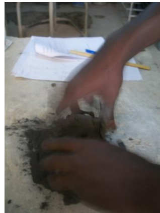
Plate 7: Blending ironfilings into clay by kneading
