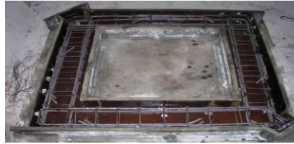
Fig 3: Details of reinforcement in the frame
