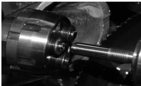
Fig.4. (a) Cylindrical rolling with two rollers (b) Direction of roller rotation
