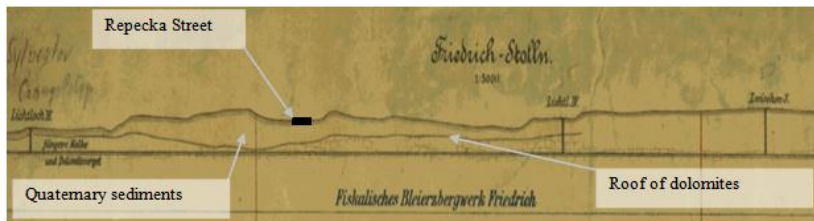
Fig.6. Cross section of the Frederick's drainage drift with the position of the roof of Triassic limestone formation and Quaternary sediments of variable thickness [1]
