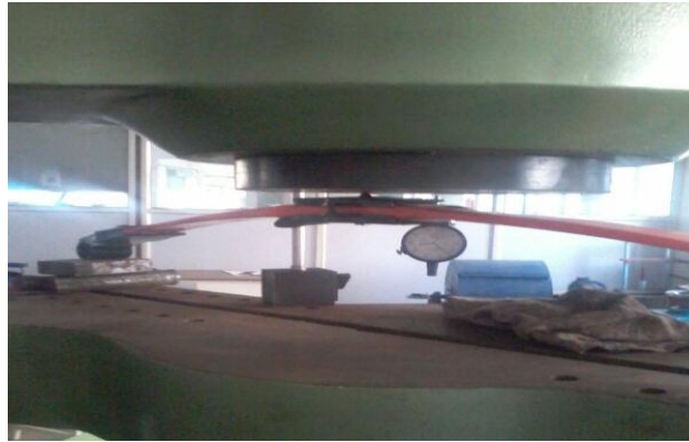
Fig.11: Static test of composite mono leaf spring
