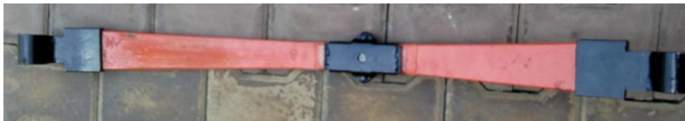
Fig.10: Leaf springs made from composite material
