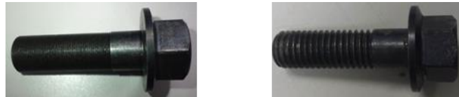
Fig. 2. (a) pitch of 0.50mm; (b) pitch of 1.75mm
