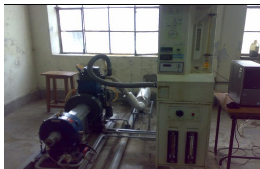
Variable Compression Ratio Engine with Loading Unit & Data Acquisition unit attached
