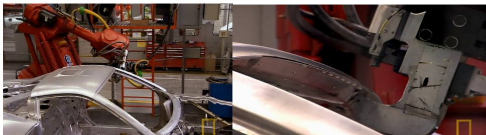
Fig 2 A& B: Robotic Spot Welding in Automotive Industry
