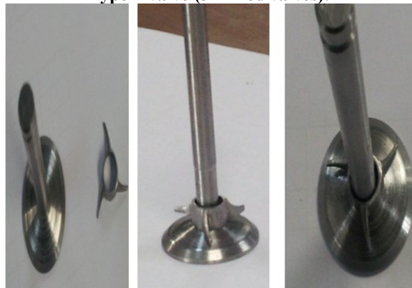
FIG-11 VALVE WITH 3 FINS
