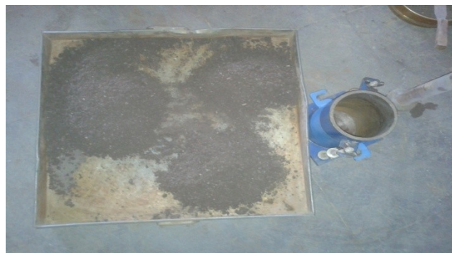
Fig 22: Sample preparation for standard compaction test
