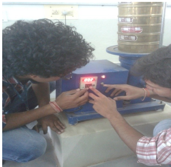
Fig.19: Operation of motor in sieve analysis
