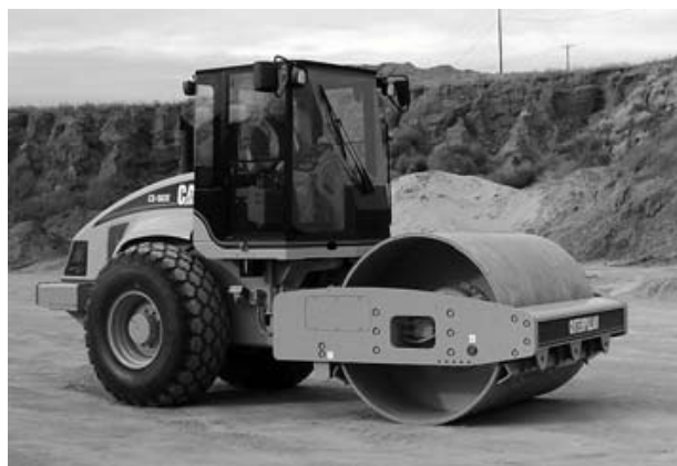
Fig 5: compaction by rolling
