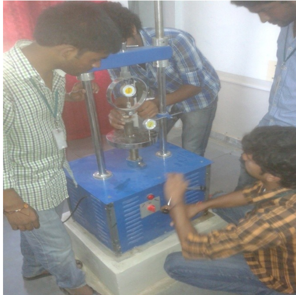
Fig 39: Operation of UCC apparatus
