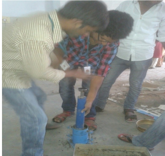
Fig 23: Compaction of soil
