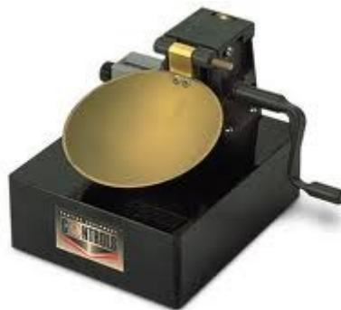
Fig 21: casagrande liquid limit apparatus
