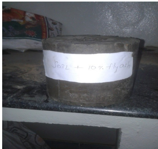
Fig 29: Soil sample mixed with 10% fly ash
