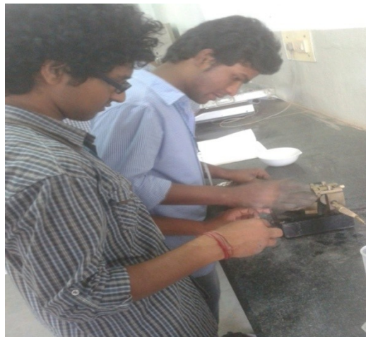
Fig 20: Casagrande liquid Limit Experiment
