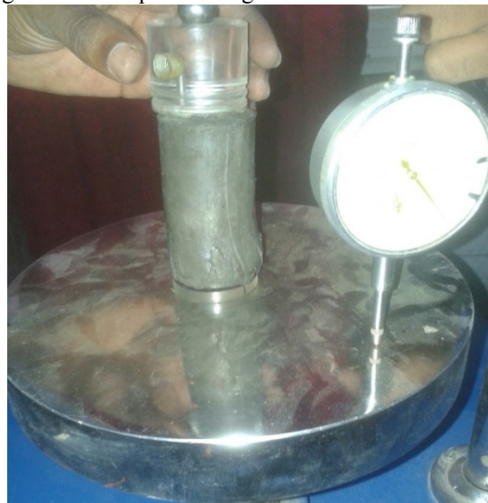
Fig 36: Arrangement of dial gauge
