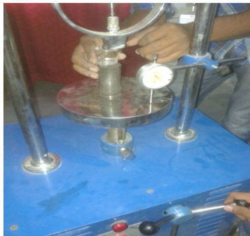
Fig 35: Arrangement of soil sample for UCC test
