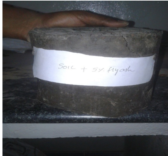
Fig 26: Soil sample mixed with 5% fly ash
