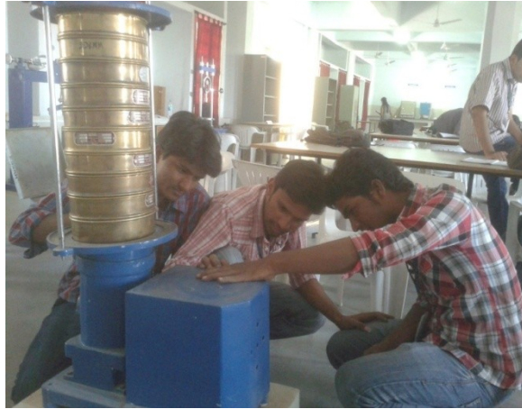
Fig 18: sieve analysis test
