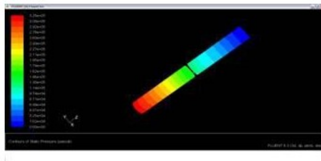
Fig. pressure lost after 2.5 seconds in TANDEM MASTER CYLINDER along with seal and leak in TANDEM MASTER CYLINDER for 5 bar
