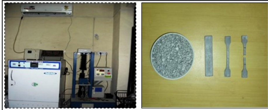
Figure 12. Uniaxial tensile test setup and test specimens by ASTM D638 standard
