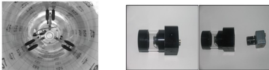
Fig 10. (a) Image Acquisition Test pipe [17] (b) CCD Camera and Lens System
