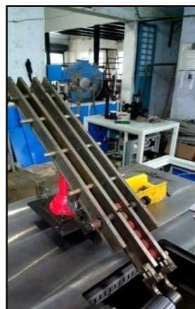
Fig. 6.3 Actual Photograph of Cot Guiding Chute
