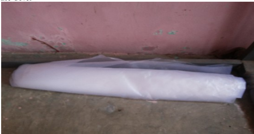
Fig 2.2 Polyethylene green house cover
