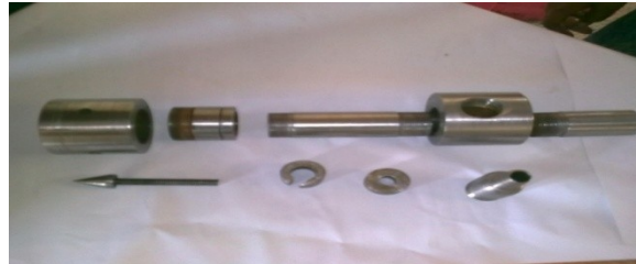
Plate no::2.8 PARTS OF VORTEX TUBE
