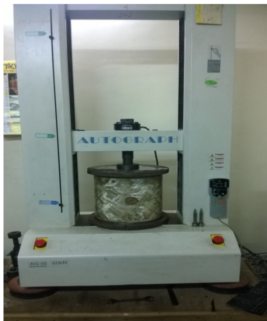
Final set up for buckling test
