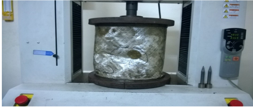
Buckling modes of the shell
