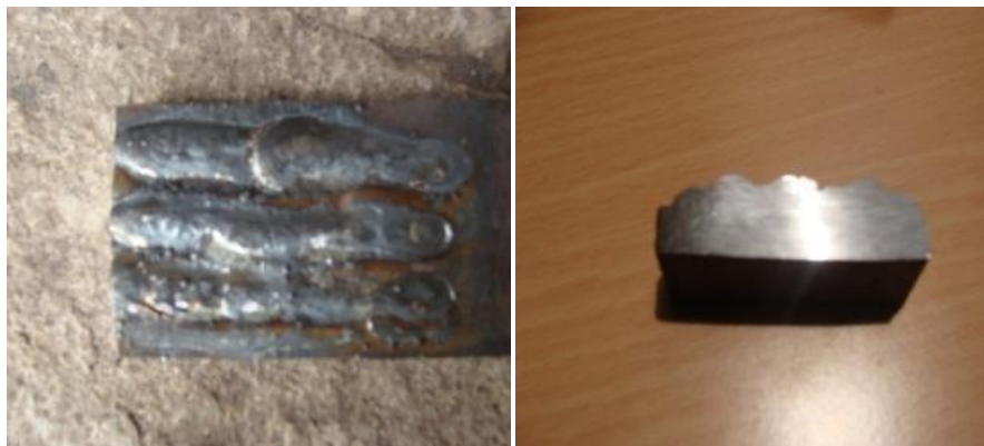
Figure: 2 showing cutting section of the hardfaced plate
