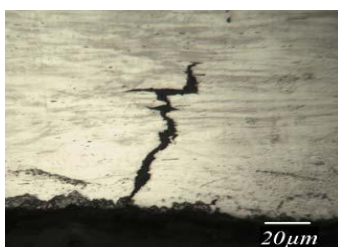
Fig.4: 316 tested in 25 MPa H 2 at 20°C showing martensite ahead of a crack tip [5]
