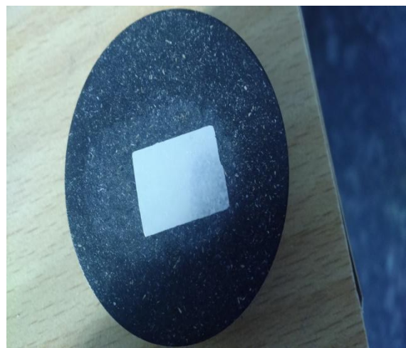
Fig.8 shows the etched sample for SEM analysis
