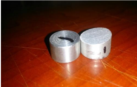
Fig.5 shows the wear samples before and after testing
