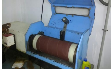
Fig.6 shows the drum type wear apparatus
