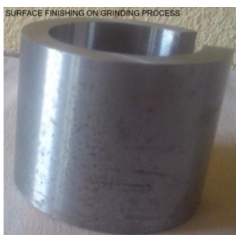
Figure 3 Surface Finishing on Grinding Process
