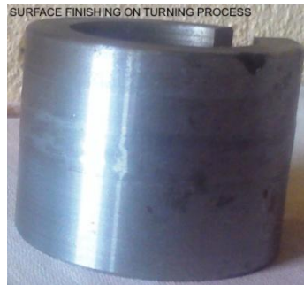
Figure.4 Surface Finishing on Turning Process
