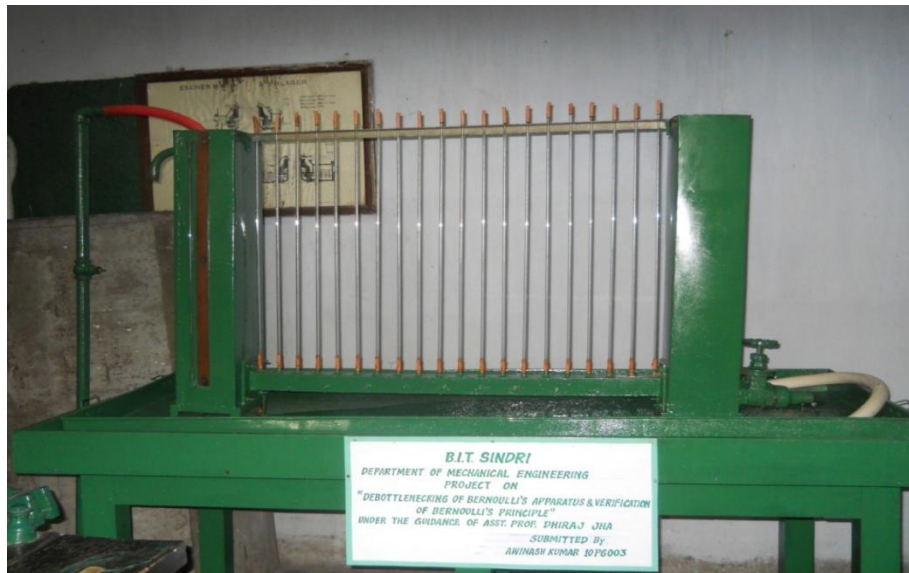
Figure: 3.2 Experimental set up of Bernoulli's apparatus at BIT Sindri Hydraulic Machines laboratory
