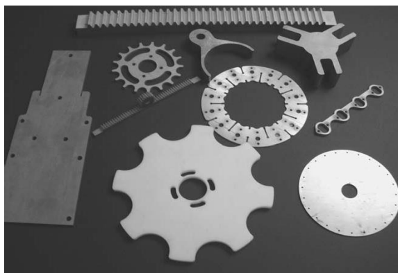
Fig. 8 Automobile parts made by AWJM
