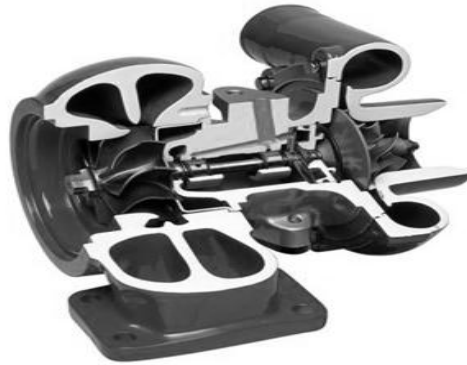
Fig 6: Turbocharger cut-away highlighting the twin-entry volute geometry, allowing differently pulsed exhaust gases to remain separate [35]
