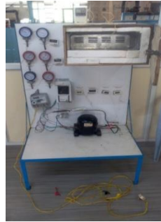
Fig 3.1 : Vapour compression refrigeration system
