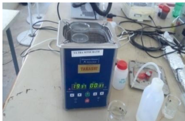
Fig 2.1 : synthesis of nanofluid in Ultrasonic vibrator
