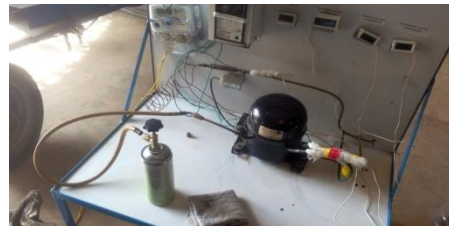
Fig 4.2 : charging of refrigerant R134a into the system
