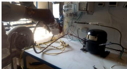
Fig 4.1: nanofluid is inserted into the compressor
